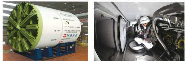
Fig. 3 Shield machine for the southbound
