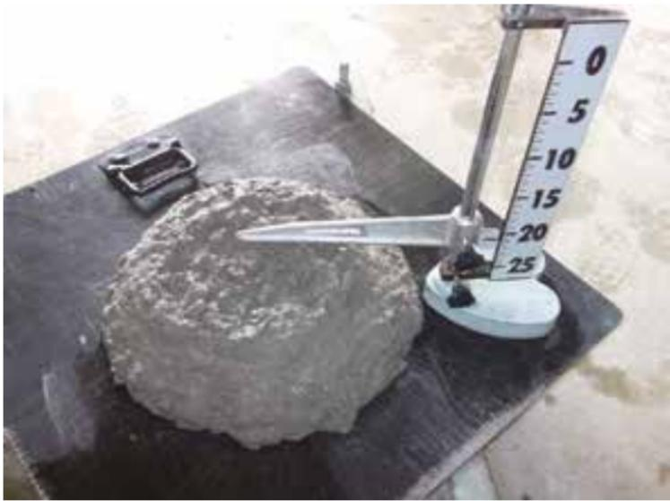
Photo 1 External view of high compactability concrete
