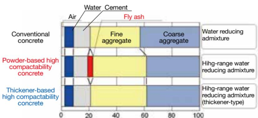
Fig. 1 Conceptual diagram of the ratio of ingredients of various types of concrete
