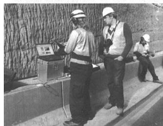
Vibration monitoring equipment in the Norfolk Tunnel
