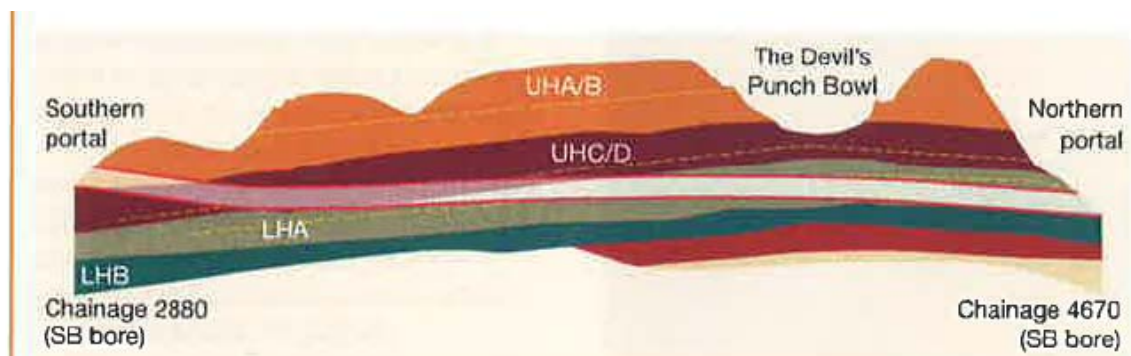
Above: Simplified longitudinal section response to tunnel monitoring and geological mapping information (figure 3).
