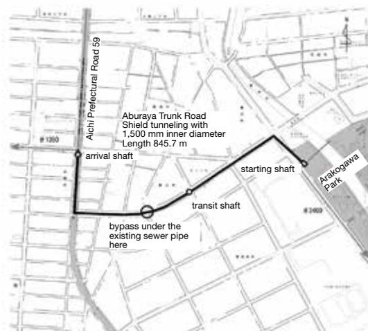
Fig. 1 Overview of Construction
