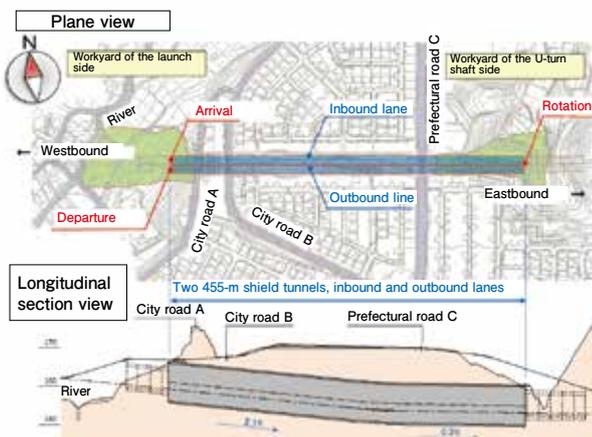
Fig. 1 Plane view, longitudinal section view
