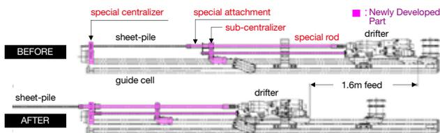
Fig. 2 Sheet-pile Installation Device
