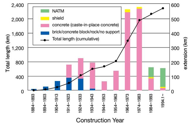
Fig.-4.2 Number of tunnels constructed by the seven JR companies (former national railway) by year (as of 2002)
