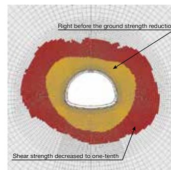
Fig. 3 Change in plastic zone due to bedrock degradation
