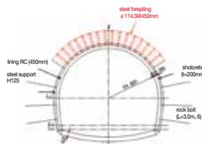
Fig. 4 Support Pattern where Steel Forepiling was Used
