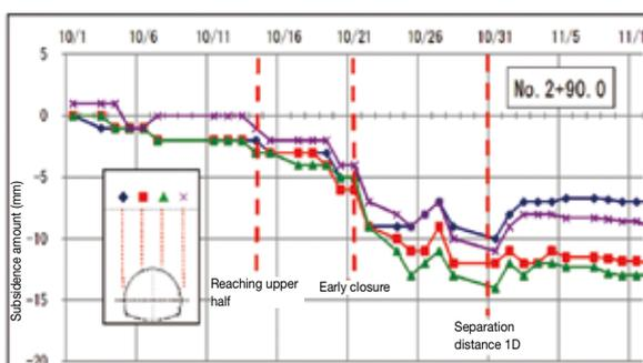
Fig. 2 City road surface subsidence measured
