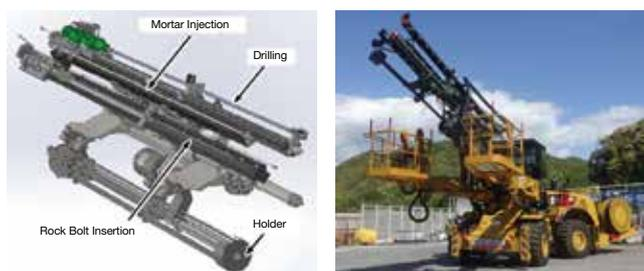
Fig.1 Composition of the Rock Bolt Placement Boom
