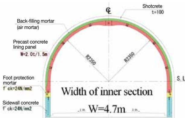
Fig. 1 Cross-section view of the evacuation tunnel
