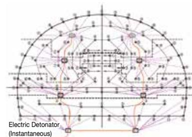
Fig. 5 Controlled Blasting using a Detonator with a Fuse Tube
