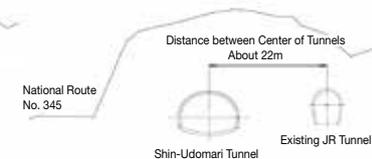
Fig. 2 Cross-section of Existing Railway Tunnel at its Nearest Point
