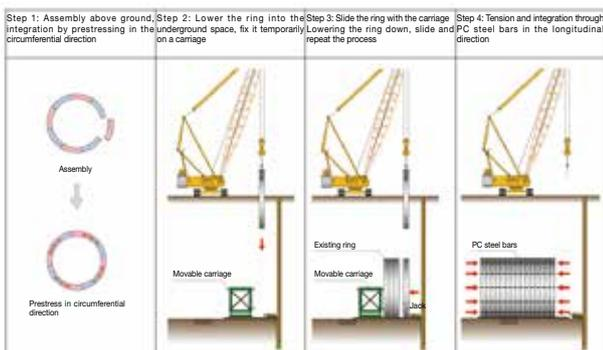
Fig.1 Construction process
