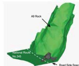
Fig. 4 Results of Rock Fall Simulation
