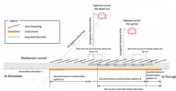
Fig. 3 Excavation Plans Directly under Existing Tunnel
