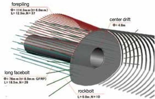
Fig. 4 Summary of Countermeasures to Prevent Landslides
