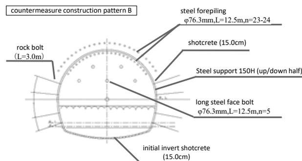
Fig. 4 Excavation Pattern
