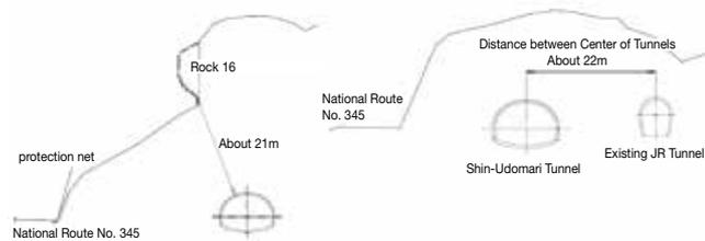
Fig. 1 Location of Rock in Danger of Falling 16
