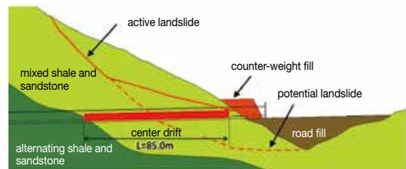
Fig. 3 Geological Profile of South Site Portal
