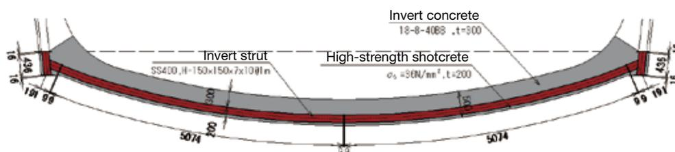
Fig. 1 Invert Reinforcement
