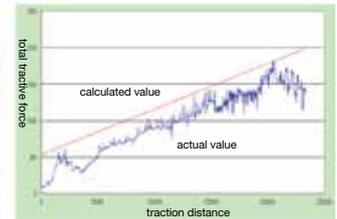
Fig. 1 Graph plotting the relevance of actual tractive force to distance (upper floor element)
