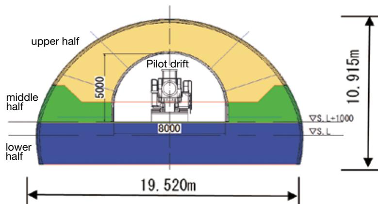
Fig. 1 Pilot Drift and Three division excavation
