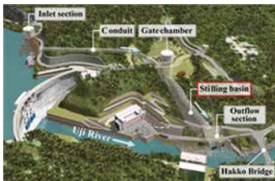
Fig. 1 Layout of tunnel-type discharge facility
