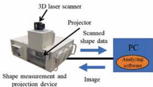
Fig. 1 Configuration of equipment for the system
