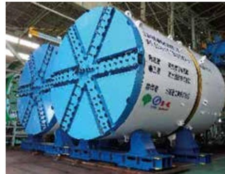
Fig. 2 H&V shield machines
