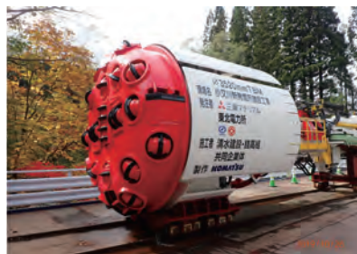
Photo 2 External view of the Φ3.52m Open-type TBM
