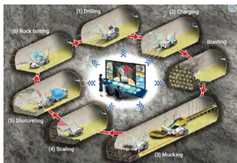
Fig. 1 Kajima's concept of “A4CSEL for Tunnels”
