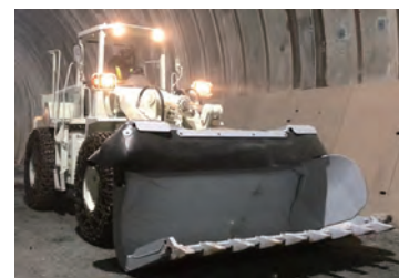
Photo 1 Wheel loader equipped with Slide Loader™
