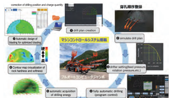
Fig. 1 Workflow of Automatic Blasting Design and Construction System for Optimized Blasting
