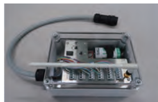
Fig. 2 Data logger with LPWA
