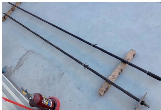
Fig. 2 6m joint rock bolt
