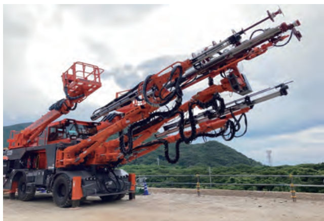
Fig. 1 “BOLTINGER”, a special driving machine for rock bolts (with 2 booms and 2 baskets)
