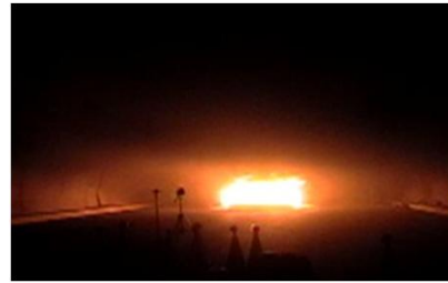
Photo-1 Fire experiment inside tunnel (approx. 3 min after ignition)
