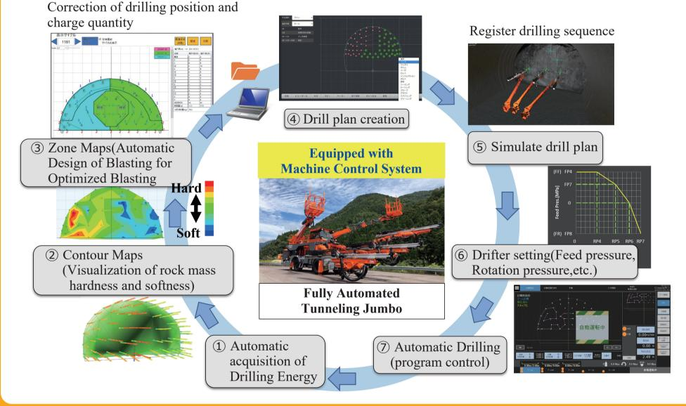
The system automatically designs blasting patterns using rock strength evaluated from the drilling energy obtained by the fully automated Jumbo. Subsequently, the Jumbo automatically perforates using the designed blasting pattern.
