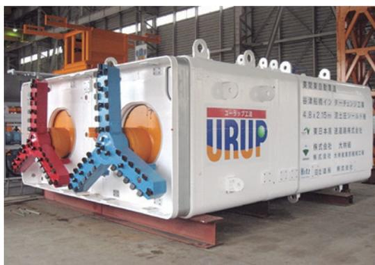
Photo 1 Closed type high, density slurry shield method
