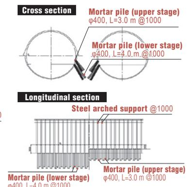
Fig. 3 Displacement control with mortar piling
