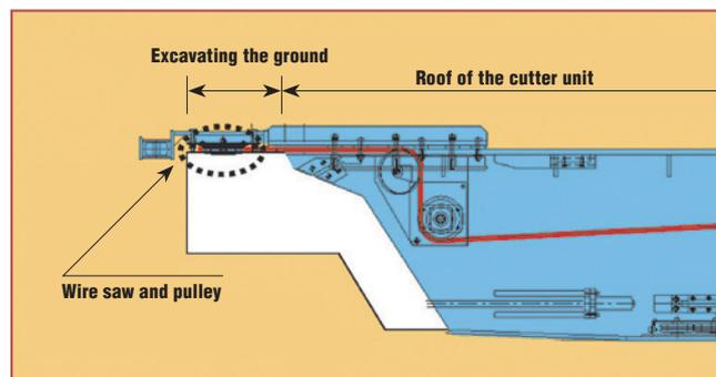
Fig. 2 Replacement of the ground cutting system
