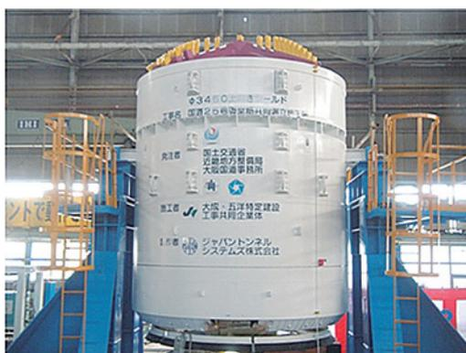
Photo Upward shield machine
