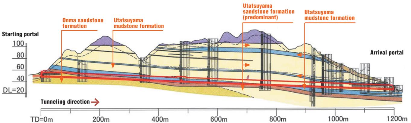
Fig. 1 Geological profile of the 2nd Utatsuyama Tunnel
