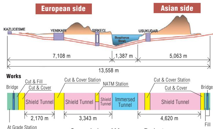
Fig. 2 General plan of Marmaray Project
