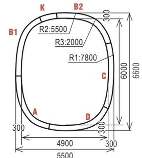
Fig. 2 Combined-circular shield tunnel section (single track)
