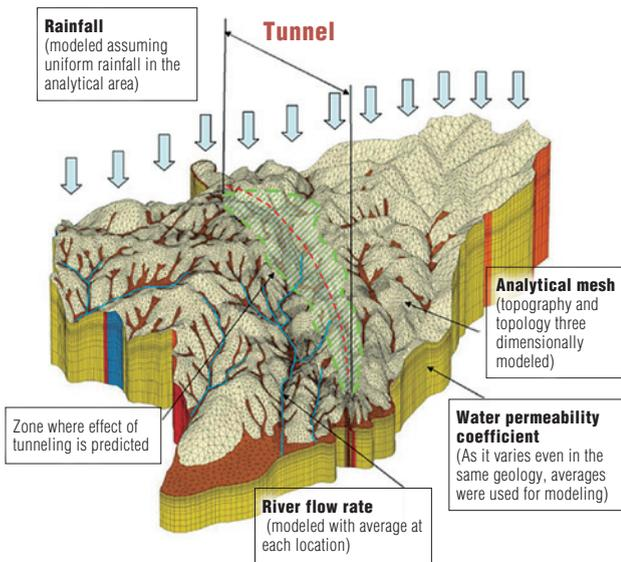
Fig. 1 Schema of the 3D infiltration analytical model
