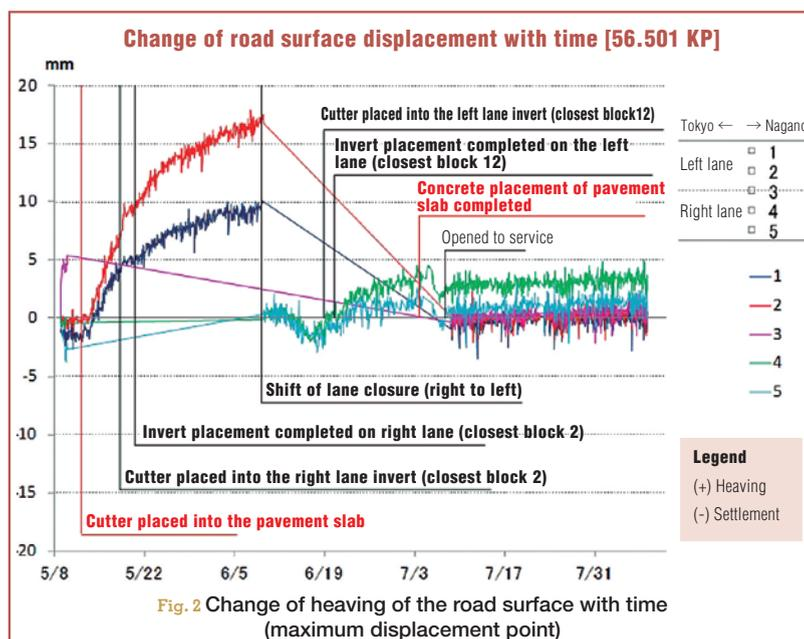
Fig. 2 Change of heaving of the road surface with time (maximum displacement point)
