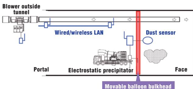
Fig. 3 General diagram of the ventilation system
