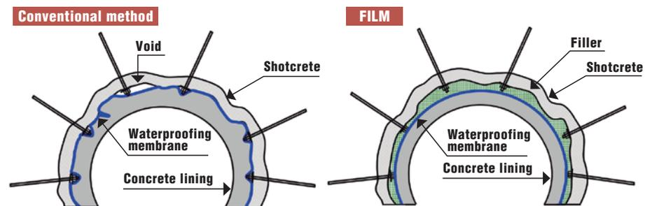
Fig. 2 Concepts of conventional lining method and FILM
