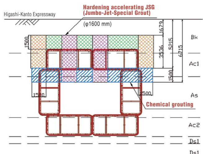
Fig. 1 Sub-section shield tunneling and ground improvement
