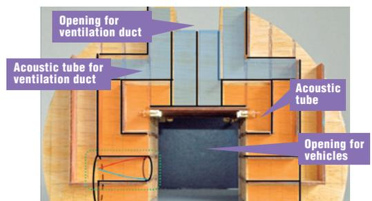
Fig. 3 Schematic diagram of the silencer
