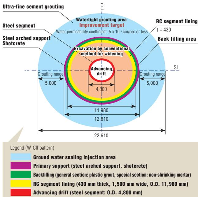
Fig. 1 Cross section of the waterproof structure
