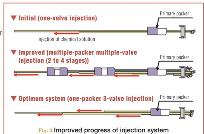
Fig. 3 Improved progress of injection system
