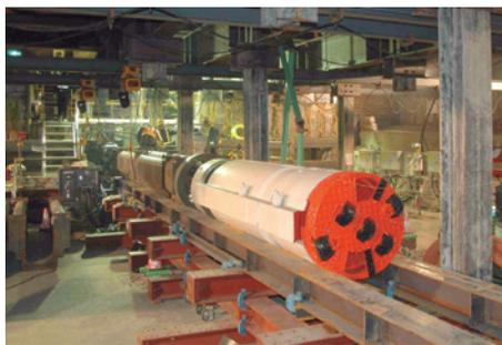
Photo 1 Pipe roof drilling machine
