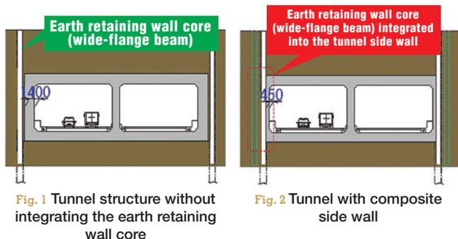
Fig. 1 Tunnel structure without integrating the earth retaining wall core
