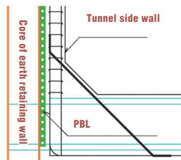
Fig. 3 Structure of the side wall section
