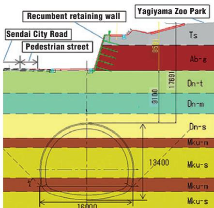
Fig. 1 Geological section of the large-section segment of the asymmetrically pressured topography
