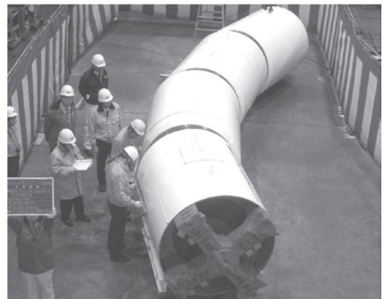
Photo 1 Main assembly of the excavator
