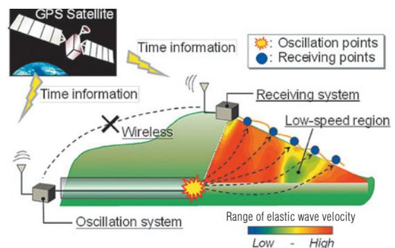
Fig. 1 Schematic diagram of the survey system
