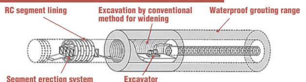
Fig. 2 Construction method of the watertight structure zone
