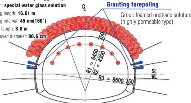
Fig. 2 Support pattern using various auxiliary methods
