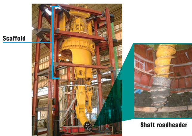
Fig. 2 Photo of the excavation apparatus (roadheader and scaffold) used for sinking a shaft.
