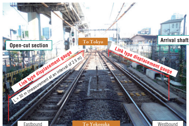
Photo 3 Track displacement measurement at the railway track crossing point
