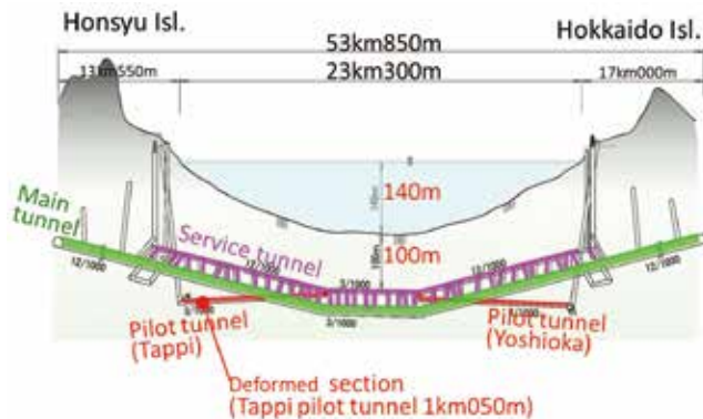
Fig. 1 Outline of the Seikan Tunnel
