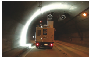
Photo 1 Taking images of the lining surface
