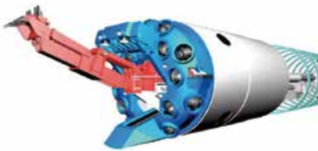
Fig.2 Conventional tunneling mode for soft ground excavation
